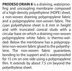
PRODESO DRAIN 8 is a draining, waterproofing, uncoupling membrane, which guarantees the vapour management with a thickness of 8 mm. It does not require expansion joints in the screed before the installa- Using PROBAND KOLL AB, bi-component tion of ceramic and natural stones.
